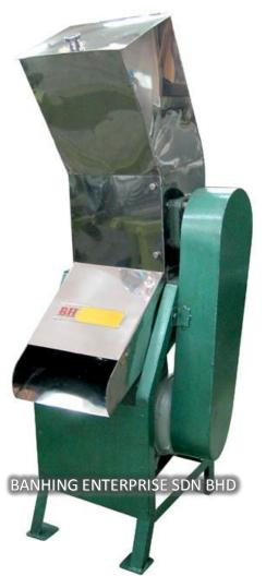
The Elec. Ice Crusher are designed for high performance. They can be used for crushing ice into small pieces, The machine work smoothly and reliably. All the machine parts & body in contact with ice or food are made of stainless steel or their surfaces are specially treaded in conformity with Chinese Hygiene Standard and mild steel structure.
